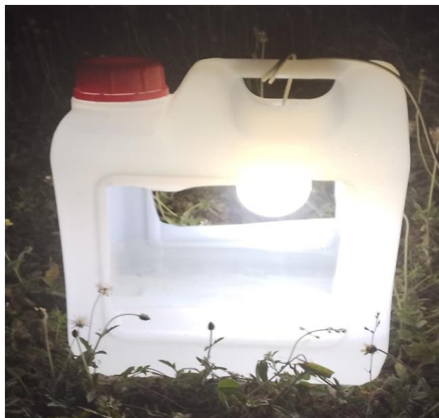
Plate 1: Constructed white light trap for nocturnal insects
